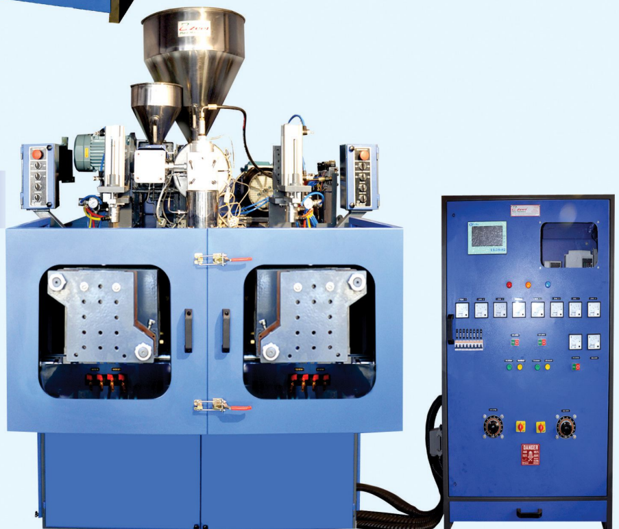
1000 ML Double Station V- Strip Plastic Extrusion Blow Moulding Machine
